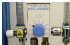
NEO 2 Air/O 2 Blender (PN 12368A70) It allows having a settable percentage O 2 on two outputs with different flow rates: 3 l/min or 15 l/min
